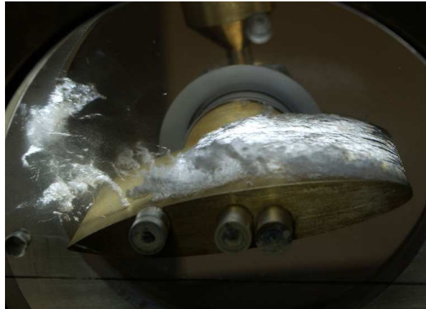
FIGURE 1.1: Sheet cavitation on 2D hydrofoil. Photo taken by Foeth.
