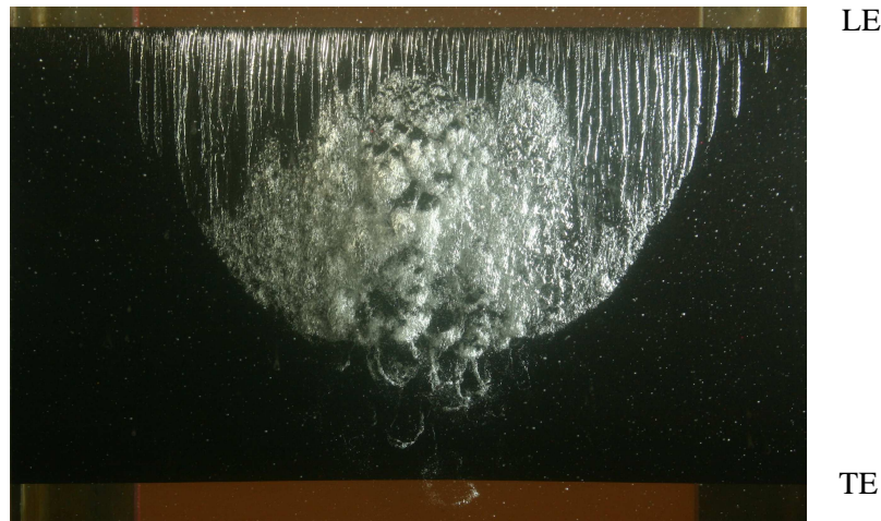
FIGURE 2.6: Top view of sheet cavitation on 3D Twist11 hydrofoil obtained from Foeth [66]. Flow is from top to bottom, LE is leading edge, TE is trailing edge.
